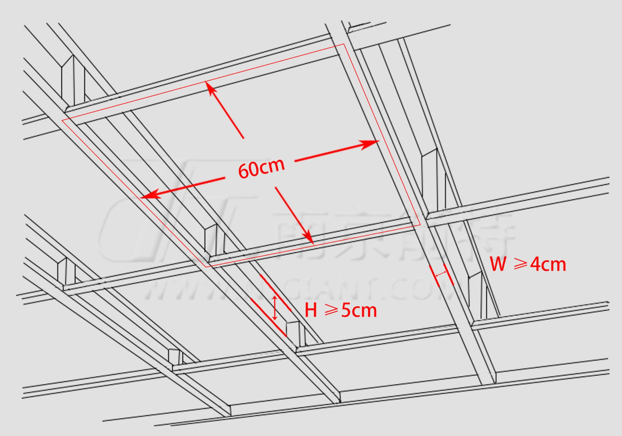
Before intalling the star panel, builing wooden frames is necessary. Frame size Hight: 2CM Width: 4CM
